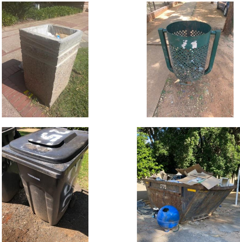
Figure 16. Main observed type of containers. (a) Concrete 0.118 m³ (b) Metal 0.118 m³ (c) Plastic 0.240 m³ (d) Skip 4 m³
