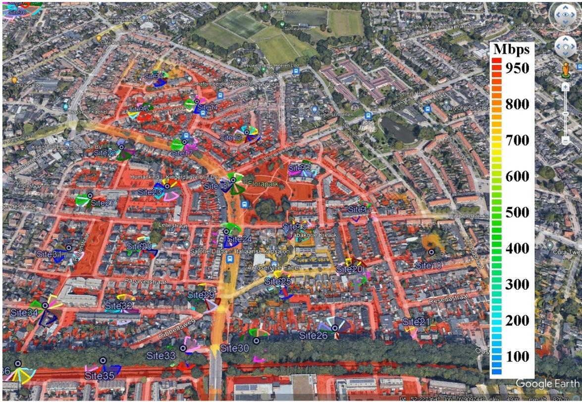
Figure 41. User Throughput prediction in the mmWave portion of the network.
