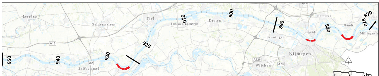
Figure 4: Rkm along the Waal with the fixed layers and bed groynes denoted in red and domain transitions denoted with the thick black lines (adapted from Esri Nederland & Sweco Nederland, 2019).
