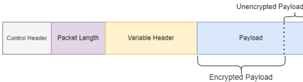
FIGURE 3.5: MQTT Protocol Header Structure and Payload Encryption
