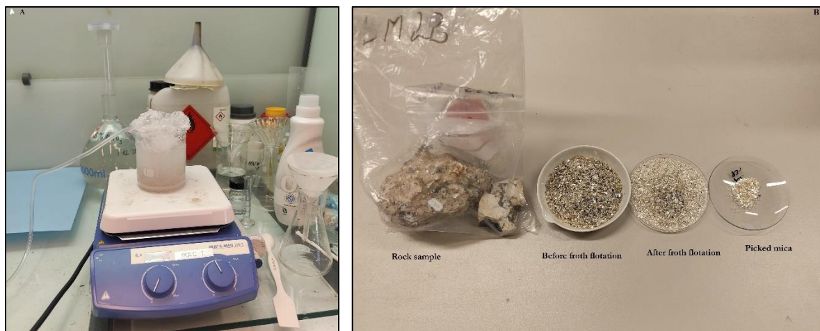
Figure 2.2: Shows the froth flotation technique to extract mica minerals (A) and the rock sample before and after the flotation technique (B).
