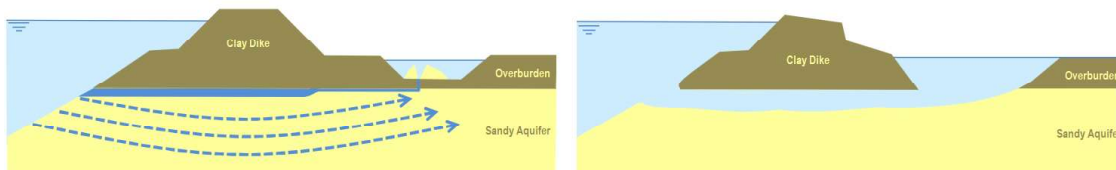
Figure 3.4: 1. After the entry point has been reached, the widening process starts from the upstream side. 2. After the widening process reaches the exit point, the soil beneath the embankment quickly fails, resulting in a dike breach (de Bruijn, 2013; 't Hart, 2018)
