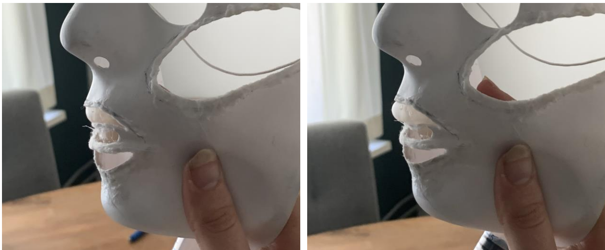
Figure 18: Effect of subtly inflating the upper lips
