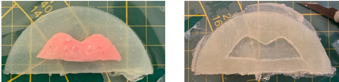
Figure 16: Process of creating an air chamber using polymer clay
