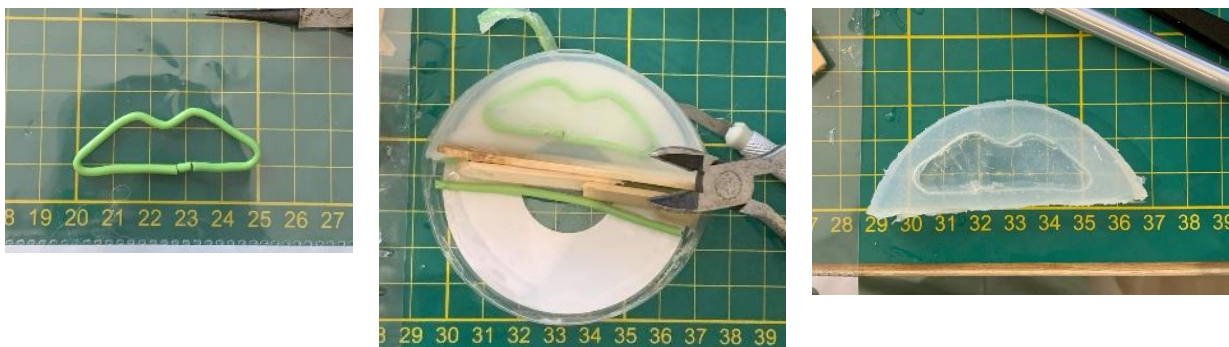
Figure 15: Process of creating air chambers using tie wire
