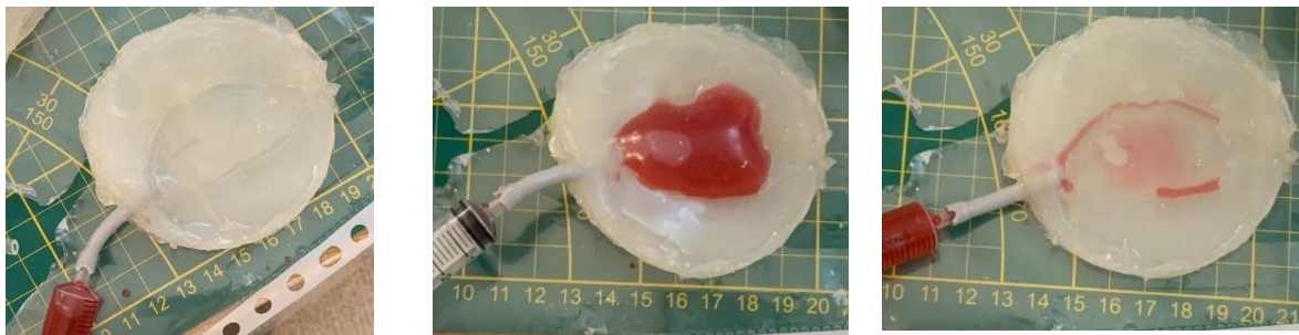
Figure 19: Colored liquid injection into a silicone piece. Left: Prior to injection, Middle: Complete injection of liquid; Right: Removal of liquid from silicone.
