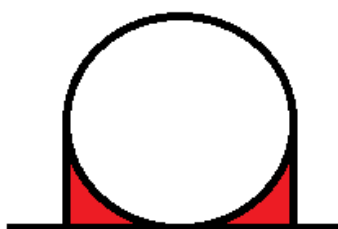
Figure 19: the measured volume of a bead (sphere) with the volume in red that is measured but not present
