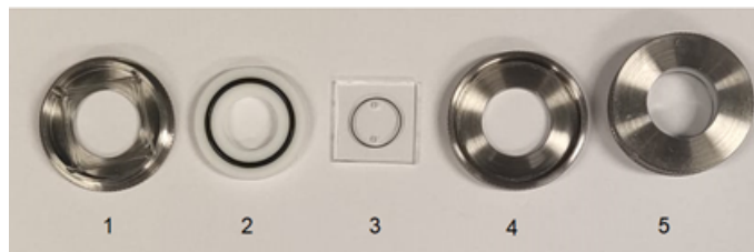
Figure 5: Parts of the metal chamber for the samples. 1,4 = casing. 2 = white pressure ring. 3 = thick glass plane with pipette holes, rubber ring, and a cover slip. 5 = assembled chamber
