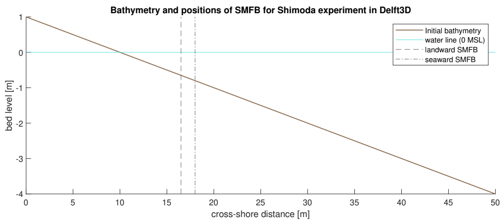
Figure 3.6. Bathymetry and positions of SMFB for Delft3D simulations in the first research phase, the waves come from the open boundary ( x=50 m)
