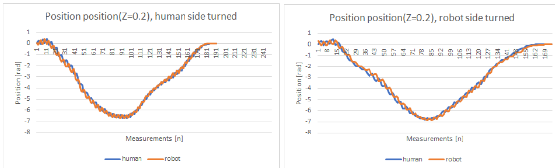
Figure 35: The response of the system at Z=0.20 in the position-position architecture
