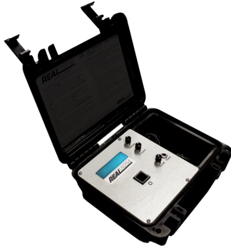
Figure 5: Van Remmen UV Transmittance Meter [24]
