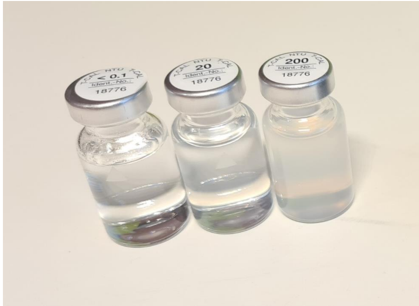
Figure 28: Control samples of known turbidity used for calibration
