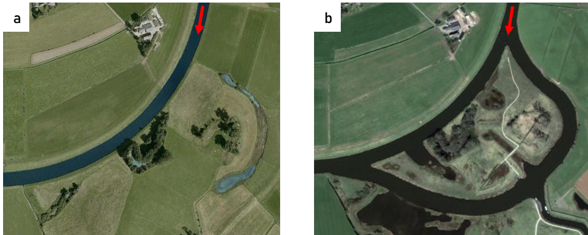
Figure 4.5. Vecht in 2005 (a) and 2012 (b) at the location of the Loozensche Linie (km 15.5-16.5). The meandering river stretch forms the main channel of the river, the old river stretch serves as a side channel with a barrier at the entrance to the side channel to guide the main flow into the meander. Red arrows indicate flow direction. Figures are adapted from Google Earth (2005 and 2012)
