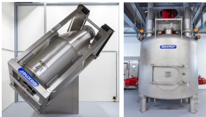
Figure 2.4: On the left, the Tumbler rotates an IBC. Right, a 10K mixer with pipes above the mixer for ingredient disposal and below for disposal of the finished product.
