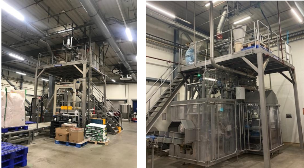
Figure 2.5: On the left, the Dinnissen packaging big bags. On the right, the Votech packaging bags
