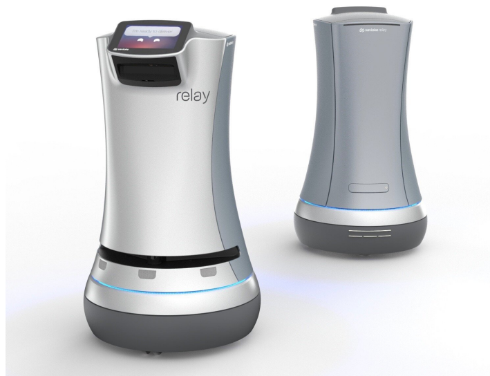
Figure 2: Savioke Relay service delivery robot. [1]
