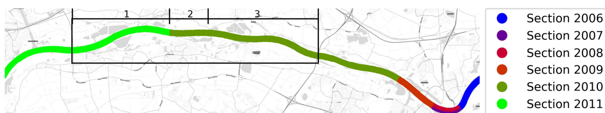
Figure 11 Roughness estimate trajectories in the main channel of the Waal. The area within the black square is the area of interest, the Midden-Waal. Note that section 2007 has a different roughness formulation due to the fixed layer near Nijmegen. The subdivision within the area of interest is needed to define the three different calibrated roughness heights in the Midden-Waal.
