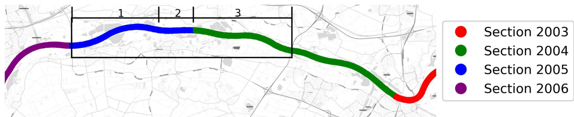
Figure 12 Spatial distribution of calibration factors sections. Note that the section names are not the same as in Figure 11. The calibrated roughness is determined by multiplying the roughness estimate with the calibration factors. The subdivision within the area of interest was needed to calculate the three different calibrated roughness heights in the Midden-Waal.
