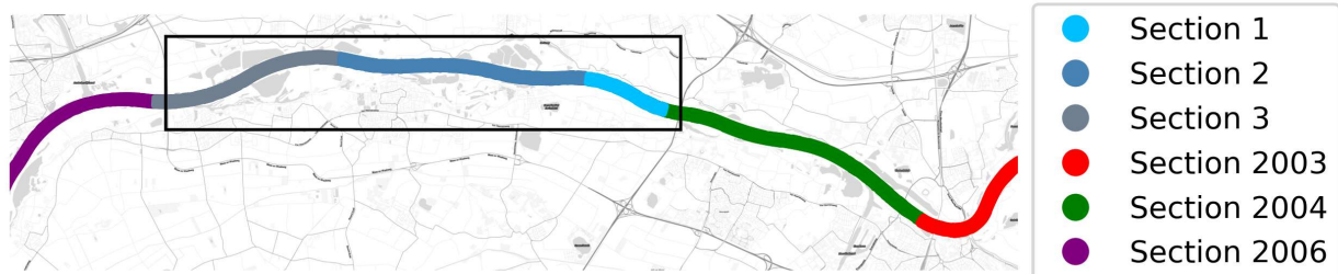
Figure 16 Modified calibration factor sections in the Midden-Waal based on trend in dune height. Roughness outside the Midden-Waal is not modified.
