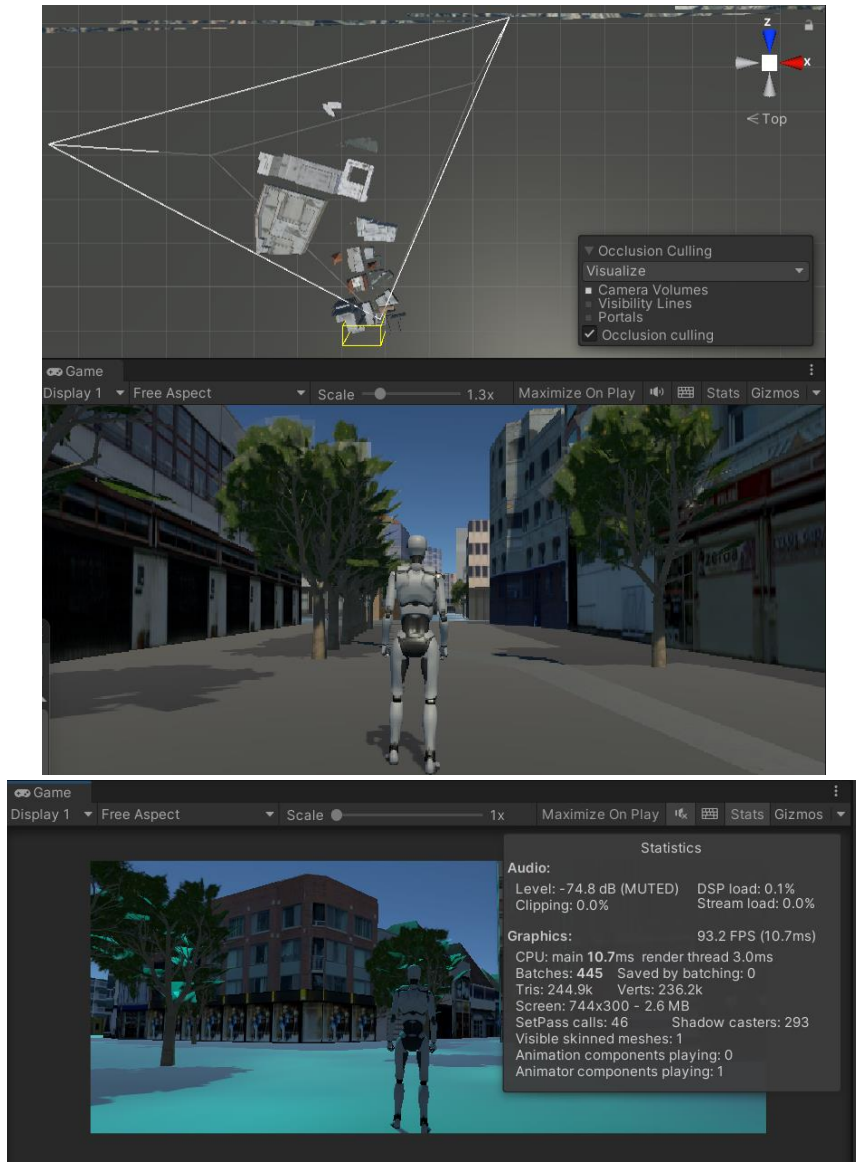
Figure 13. Occlusion culling rendering only the objects within the field of view (lines in white).
