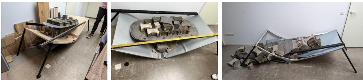
Figure 5: Glue test under continuous load, from left to right is setup 1, 2 and 3.
