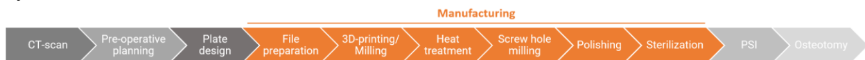
Figure 25: The workflow for manufacturing the patient-specific plate colored in orange, described within the full clinical workflow colored in gray.
