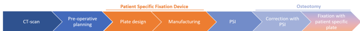
Figure 9: Proposed clinical 3D workflow in the UMCU for knee osteotomy with a patient-specific plate. Additional steps to the current workflow are colored in orange.
