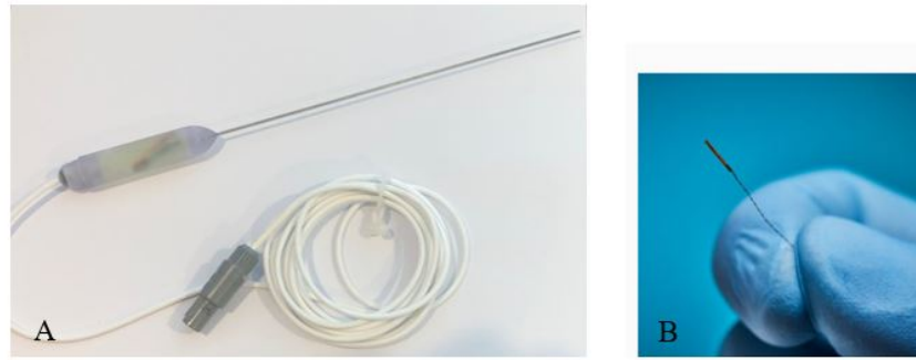
Figure 10. Design for the EM-tracked stylet (A) and the 5DOF sensor integrated into the tip of the stylet (diameter: 0.45 mm, length: 6.3 mm) (B)
