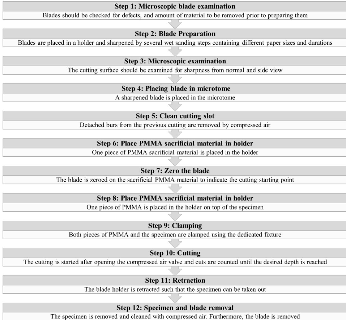
Figure 3.12: Block diagram indicating the different steps to be taken to create a pre-crack according to ESIS TC04 [50]
