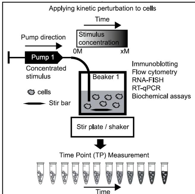
**Fig. 2.** The fluidic setup designed by Thiemicke *et al*, that enables stimulation of suspension cultures with dynamic input signals [25]. Stimulants can be added to the system but not removed, which makes the setup suitable for gradients that increase over time.
