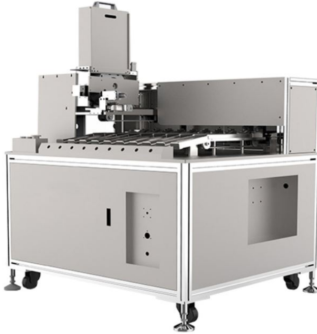
Figure 10: WinACK cell sorting machine [25]
