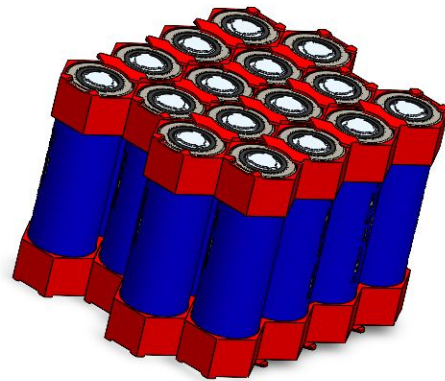
Figure 5: Combination of multiple modules form a pack
