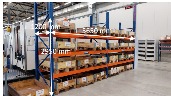
Figure 35 Storage rack with dimensions
