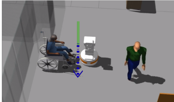
(a) Improved planner slowly going in front of the person in the wheelchair does not intrude on intimate space but takes longer time to pass in front of the wheelchair
