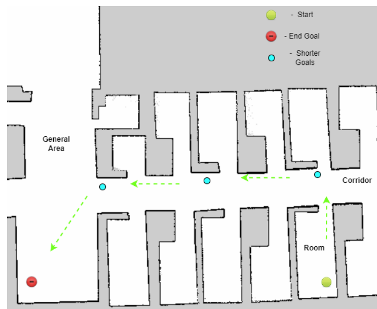
Figure 4.3: The image shows how a long path can be divided into smaller goals for the robot to achieve in order to reach the end location
