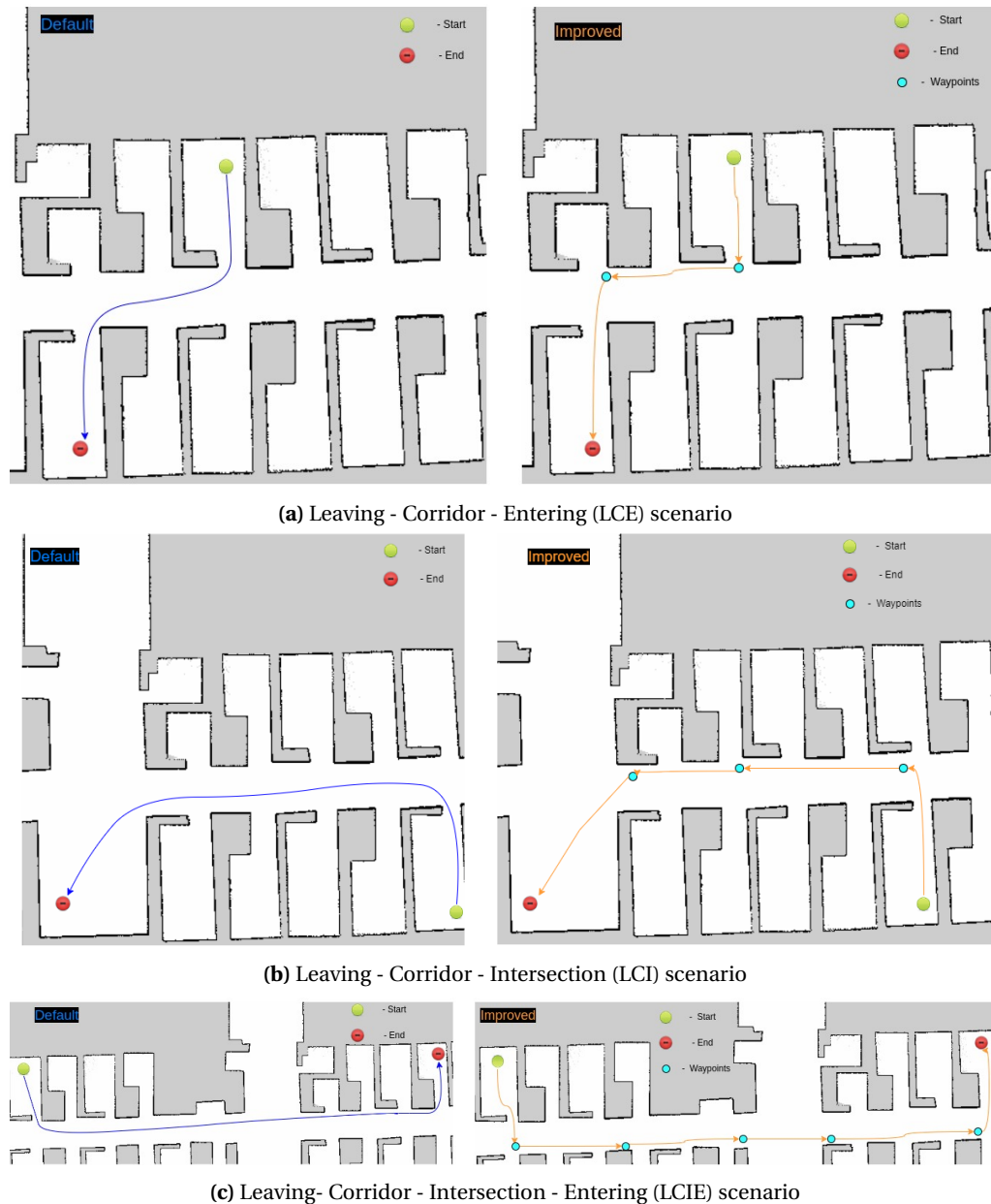
Figure 6.2: Distance comparison of the robot's travelled path from start to end location in three scenarios: LCE, LCI and LCIE. The image describes the path the robot took to reach the end goal. The difference in the distance between the start and end location changes the pattern of the travelled path
