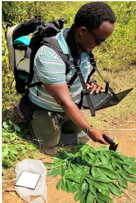
Figure 3 Spectral measurements of Casava leaf layer stack during the field campaign in Busia County, Kenya
