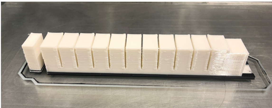
Figure 4.2: The actuator on the heated bed directly after printing. On the left the prime pillar can be seen. Also a skirt can be seen around the actuator.
