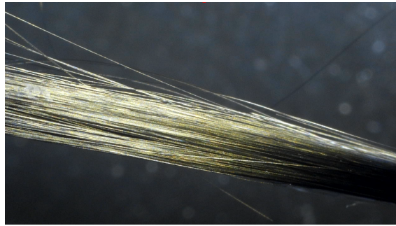
Figure C.1: Exposed fibers inside filament
