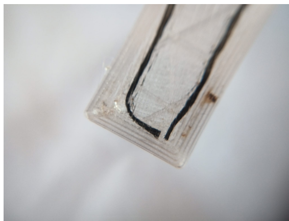
Figure E.1: Sample with one reinforced perimeter where the ends of the fiber loop are not properly connected
