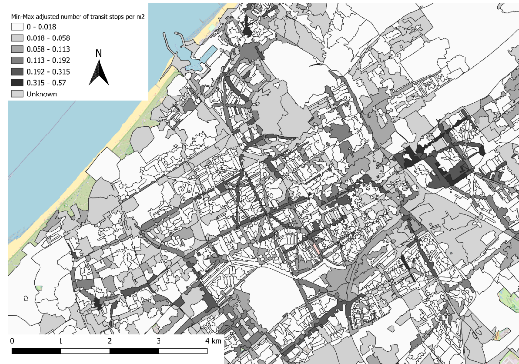
Figure 100 – Min-Max adjusted number of transit stops per m 2 per PC5 area in The Hague
