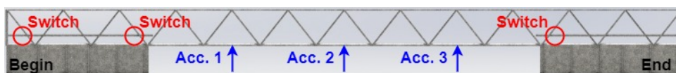
Figure 3.12: Switch and sensor locations on the experimental setup during the dynamic experiments.
