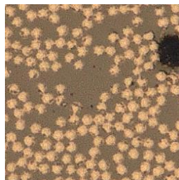
(b) Image from the sub data set “LM-PAEK 7” with void.
