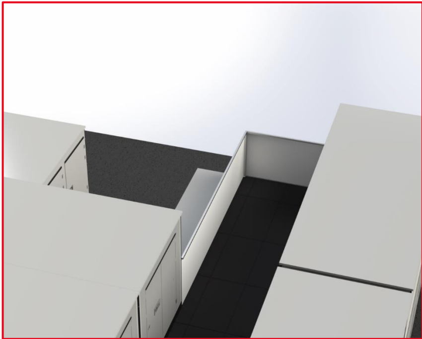
Figure 91 Railing at the corner edges of the two-story storage park
