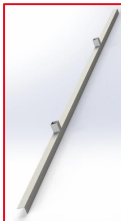
Figure 88 L-bracket with mounting points for vertical beam
