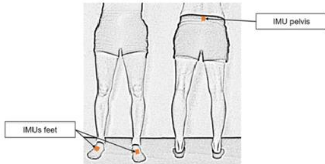
Figure 2: The placement of the three IMUs: one on the lower back, one on the left foot, and another one on the right foot. The picture has been adapted from the following source [15].
