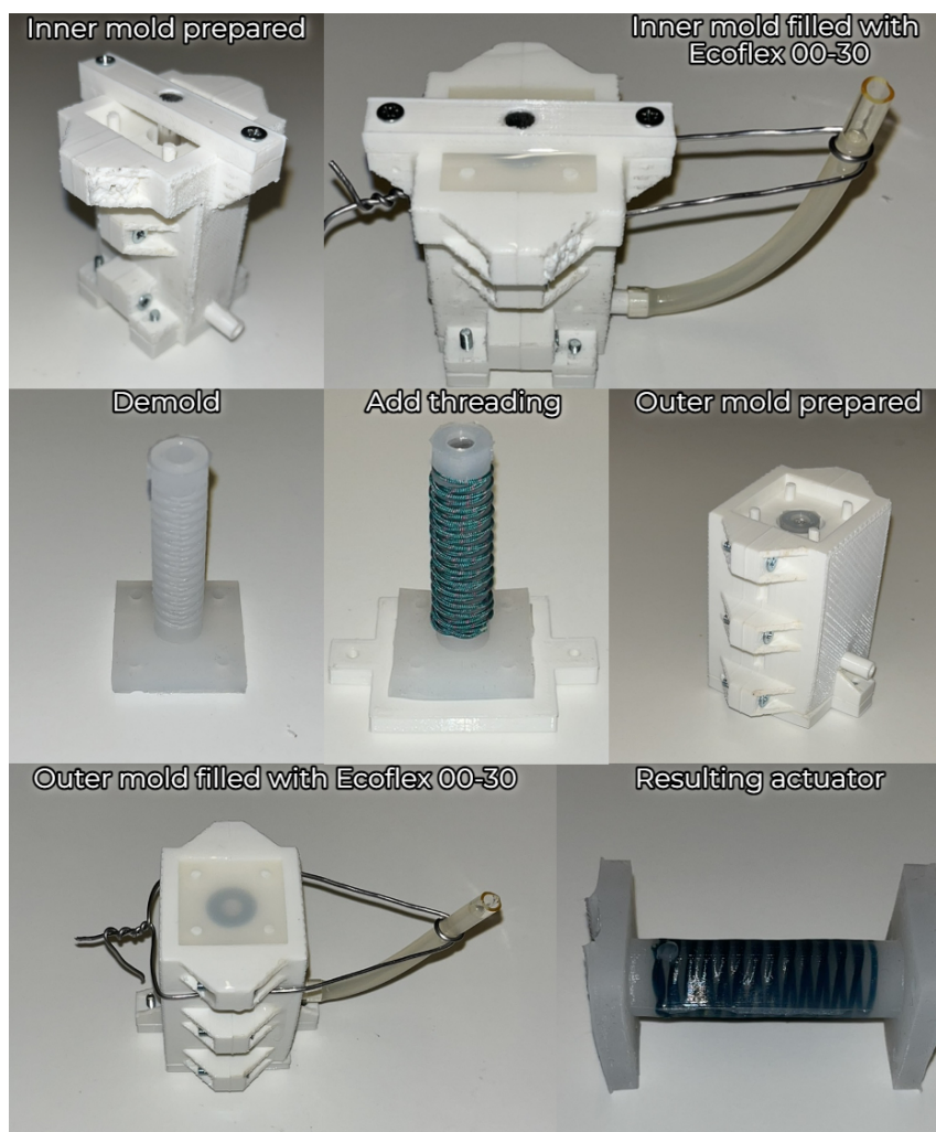
Figure 2.9: The fabrication of the given device's actuators
