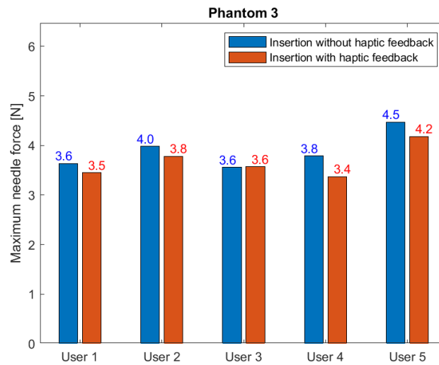
Figure 4.7: Average of the second two insertions into phantom 3. The first insertion is removed due to a problem with the phantom that caused high outliers in the case without haptic feedback.
