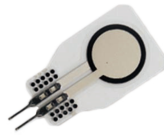
Figure A.12: The force sensor used on the haptic device. Its part number is GD10-20N [77].
