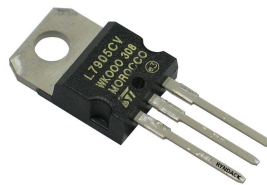
Figure A.10: The voltage regulator used to regulate the -5 V. The regulators part number is LM7905 [93].
