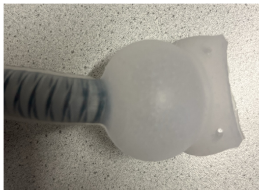
Figure 3.4: Ballooning of the actuator where threading is not constraining the actuator from radial expansion.
