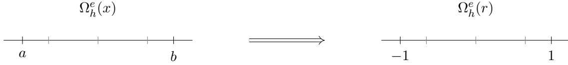
Figure 2.8: Transformation from an arbitrary 1D element \Omega_h^e(x) to a standard element \Omega_h^e(r) . The grid points are illustrated by LGL points for p = 4 .
