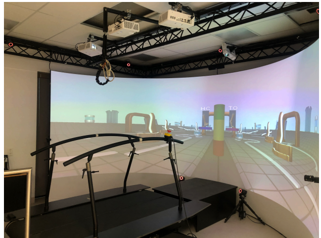
Figure 1: Gait Real-time Analysis Interactive Lab (GRAIL) including the variable-speed treadmill and harness safety hook. The virtual environment and feedback were projected on the screen.
