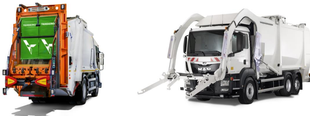
Figure 1-3. Bin Lifter and Front Loader of Terberg Dennis Eagle LTD
