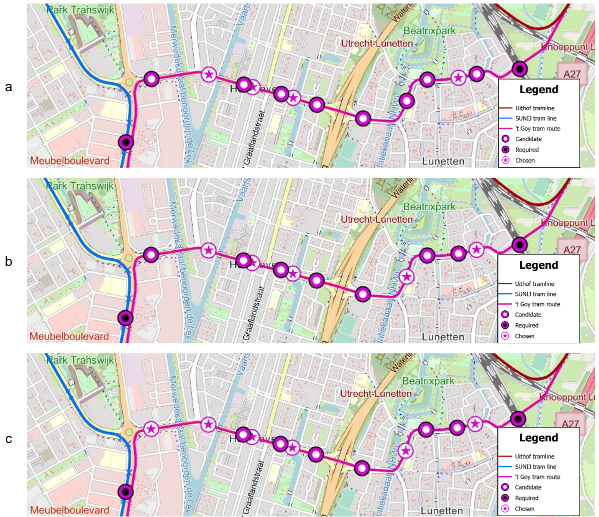
Figure 14: 6 (a), 7 (b) and 8 (c) tram stops for 10 minutes walking reach to stop locations.
