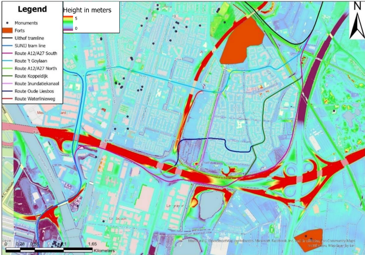
Figure 23: All considered tram routes, including elevation map: Purple ( \leq 0 meters +NAP) to Red ( \geq 5 meters +NAP) (AHN, 2022)
