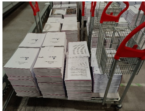
Figure 12 A book block cart used for transporting printed book blocks to subsequent workstations
