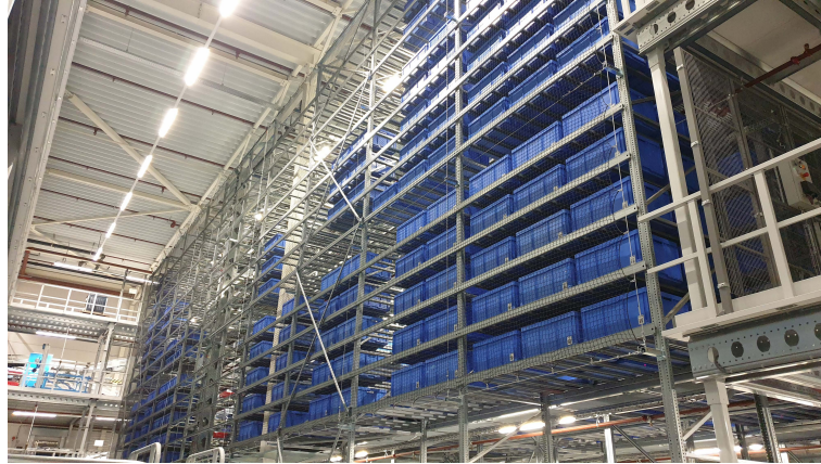
Figure 7: The Stingray, a tote buffer
