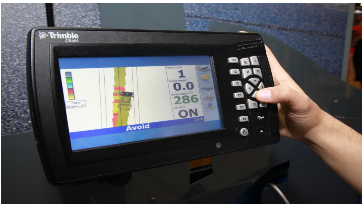
Figure 7 Trimble Compaction Control (World Highways, 2017)
