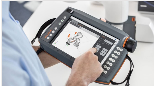
Figure 2: KUKA SmartPAD Being Used to Program and Adjust a Cobot Application
