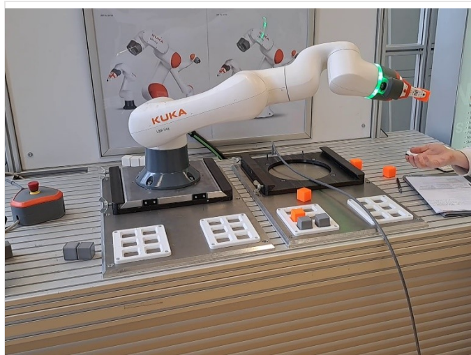
Figure 3: KUKA LBR iisy setup used for self-test
