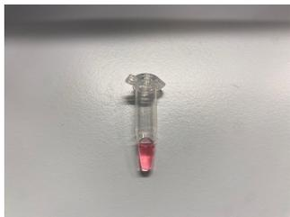
*Figure 6: Untreated AuNPs, as a reference for the colour all samples had before adding NaCl and incubating.*
