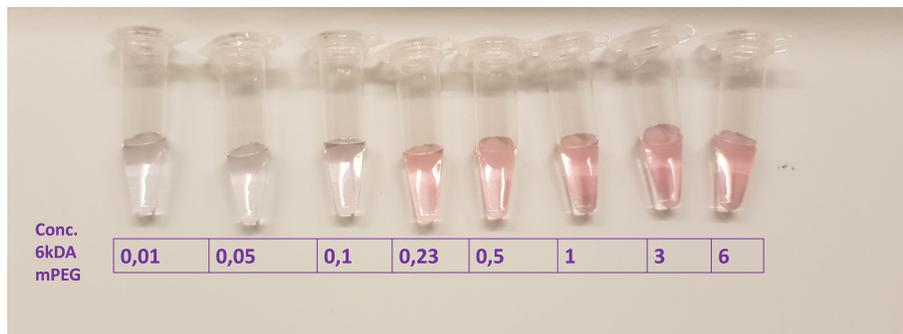
(c) The salt concentration for 6kDa mPEG was increased with as a result that with low mPEG concentrations the AuNPs dit start to coagulate.
