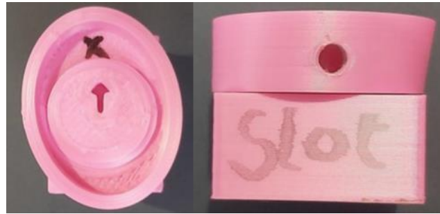
Figure 24 Best combination concept 2: -0.2mm offset and 0.25mm fillet on thread with no offset and no fillet for nut
