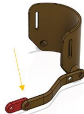
Figure 2 Triceps plate with hinge plate and an extra smaller plate for an additional pivot point
