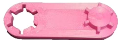
Figure 20 3D printed tool to tighten and remove the adapter in the hand (hole on the left); the guidance in the forearm (height on the right)
