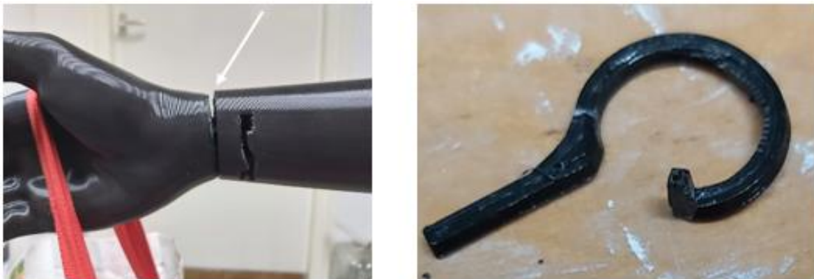
Figure 17 Testing of the combined concepts with a load of 17.5 kg for 2 hours.
