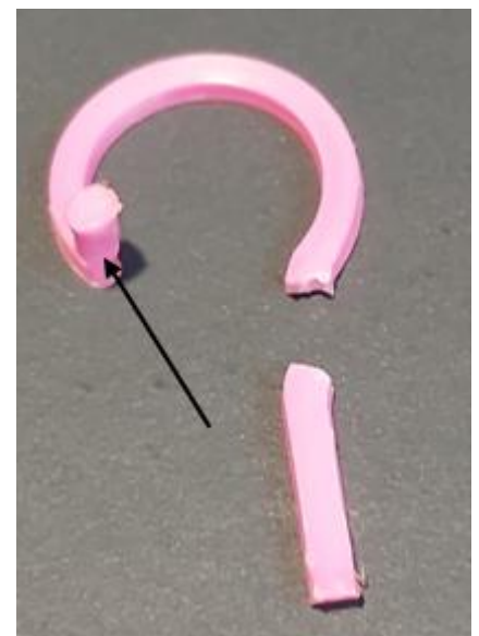
Figure 28 Torsion spring with width 2mm, 15mm diameter and 0.7 revolutions which broke due to overstressing the lever. The black arrow highlights the blob which occurs during printing with 0.4mm and 0.8mm nozzle.
