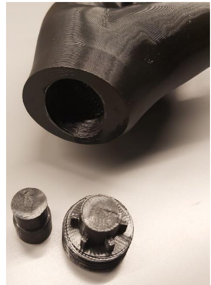
Figure 21 Broken adapter of the newly selected concept. No deformations are found in the hand and thread
