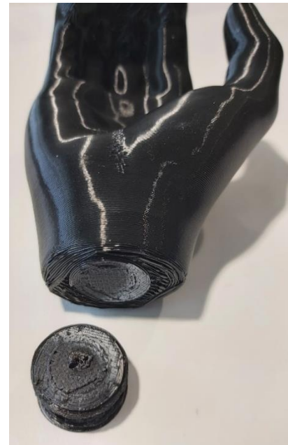
Figure 14 Testing of threaded concept. The location of breakage in the wrist adapter after an applied load of 62.9 kg.
