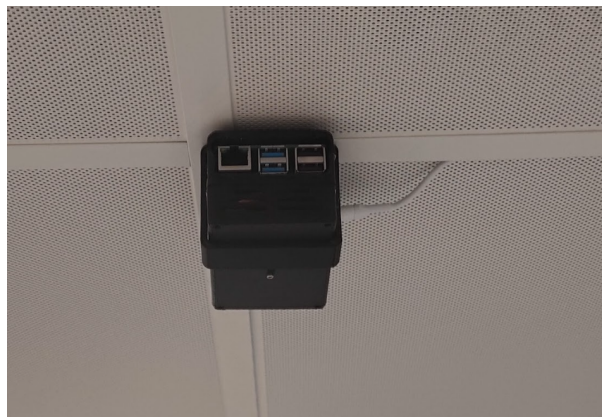
FIGURE 6.16: Case with temporary mounting attached to ceiling
