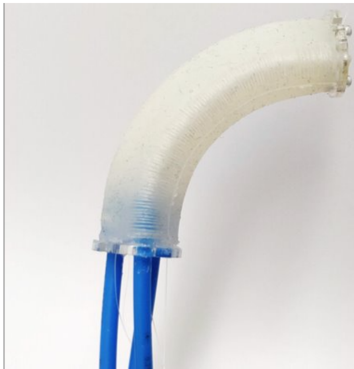
Figure 1.2: The investigated soft continuum robot. It consists of a single segment which is intrinsically actuated via three internal elastic pneumatic chambers. Therefore, its core structure is composed by four elastic elements i.e. the three soft actuators (blue rods) plus the main backbone. Hence, the investigated device constitutes a pneumatic-driven, single-segment, multi-backbone continuum robot.
