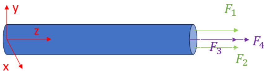
Figure 3.5: Modelled actuation in Elastica. The cosserat rod is in its initial state. If the four actuators produce forces with magnitudes F_1 = F_2 and F_3 < F_4 , the rod will elongate along the endpoint's tangent vector and perform bending in the X-Z plane.
