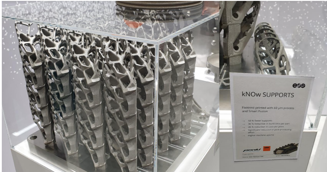
Figure 4.1: Example of motor-cross footrests printed stacked on top of each other developed in a collaboration by EOS and Pankl [80].
