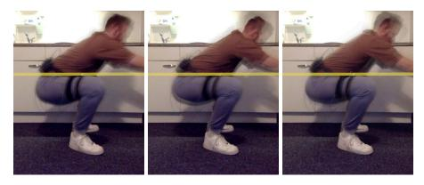
Figure 5.2: images from 3 series of 10 squats overlaid on one another to measure the squat depth sensor's accuracy
