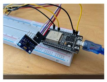
Figure 2.8: ESP-32 with an MPU-6050 gyroscope/accelerometer
