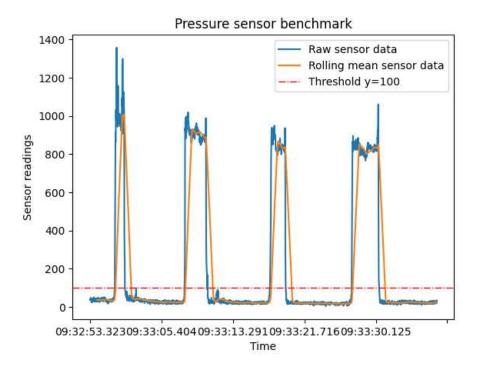
Figure 6.4: Benchmark of the pressure sensor
