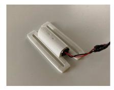
Figure 6.5: A vibration motor in its 3D-printed casing
