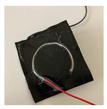
Figure 6.3: The pressure sensor made with Velostat
