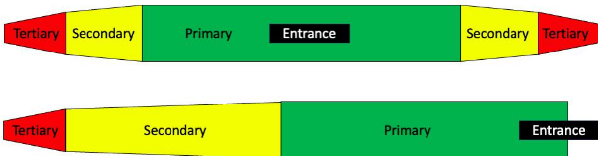
Figure 3.1: Indicative length distribution of primary, secondary and tertiary zones of two platform types [Adapted from (ProRail, 2020)]
