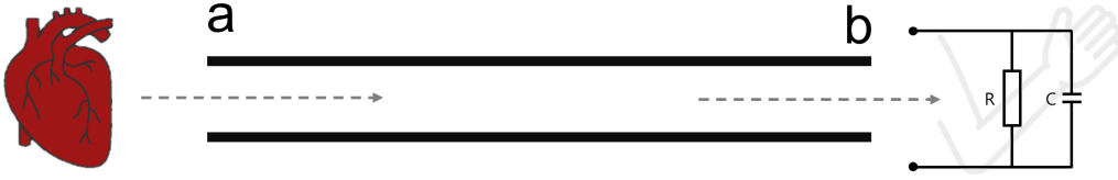
Figure 18: Schematic representation of the vessel described by the one-dimensional Navier-Stokes equations, with boundaries at the side of the LV, x = a and at the radial artery x = b .
