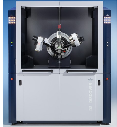
Figure 2.3: X-ray diffractometer used to analyze the oxidation state of magnetic alginate beads.
